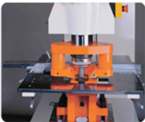
Urethane spring stripper for minimal deformation
