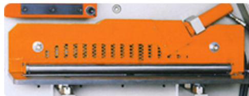
Hydraulic Holddown for Flat Shear
