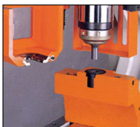
Goose-Neck Die Holder for Punching Channel Flanges & Webs
